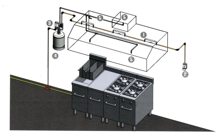
The activation mechanism trigger the system automatically or manually
